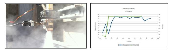
Calculations show that the ignition surface flux (ISF) was ~ 0.3 gm/cm<sup>2</sup>/sec as compared to ~ 0.2 gm/cm<sup>2</sup>/sec on previous test using the check valve. Last month, the two successful test without the check valve was with the same ISF of ~ 0.3 gm/cm<sup>2</sup>/sec but with a nozzle throat diameter of 6.0 mm. I surmise that the smaller throat diameter slowed the flow rate enough for ignition to occur while the larger throat diameter did not.
