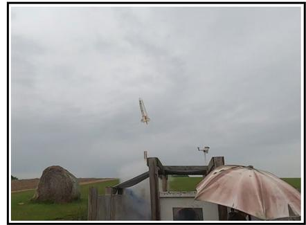
I had two launch attempts this month. I had an engine failure on the first attempt. Failure analysis showed that I did not seat the mixing chamber to the nozzle properly. I took extra care during the assembly process and the second attempt was successful.
