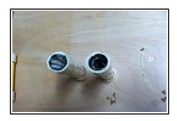
The physical analysis of the spent fuel cores introduced a new variable, stabilized vs unstabilized HTP. As shown in the picture, the fuel core on the left shows a nice even burn with PLA/KMnO<sub>4</sub> remaining in the housing. This particular rocket engine used 62.5 ml of  $\sim 85\%$  <u>stabilized</u> HTP plus 2.5 ml of ethanol. The engine burned  $\sim 6.0$  sec. The O/F ratio was  $\sim 3.3$ .
