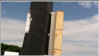
I used an iphone 5 to measure the velocity. The iphone 5 has a frame rate of 30 frames/sec. The length between each black mark is 10 cm. The first rail guide button hit the 20 cm mark at t=0 in the first frame. There are 3 frames until the first button cleared the rail guide. At 30 frames/sec, that's about 0.1 sec to clear 20 cm or 2 m/sec.
