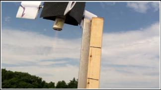
I used 50 ml of unstabilized  $\sim 90\%$  HTP plus 2 ml of ethanol for an O/F ratio of 25. Ignition occurred in  $\sim 0.3$  sec and the total burn time was about 7.3 sec. The Mk I Viper was under thrust for about 7.0 seconds. The average volume flow rate of HTPE was  $\sim 7.0$  ml/sec. The mass flow rate was about 13.29 gm/sec resulting in a propellant mass of  $\sim 93.0$  gm.
