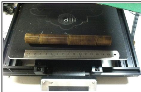
Figure 4. Assembled Fuel Core
