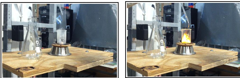
Figure 2. Drop Test of HTP on PLA/KMnO<sub>4</sub> Coupons
