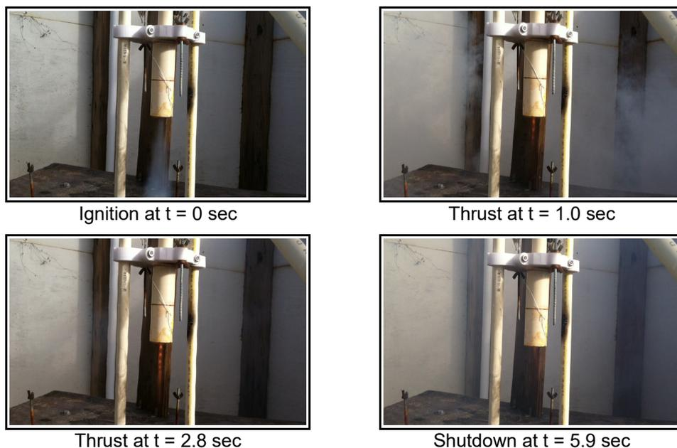
Figure 5. HTP/PLA/KMnO<sub>4</sub> Static Engine Test
