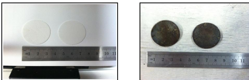
Figure 1. PLA/KMnO<sub>4</sub> Test Coupons
