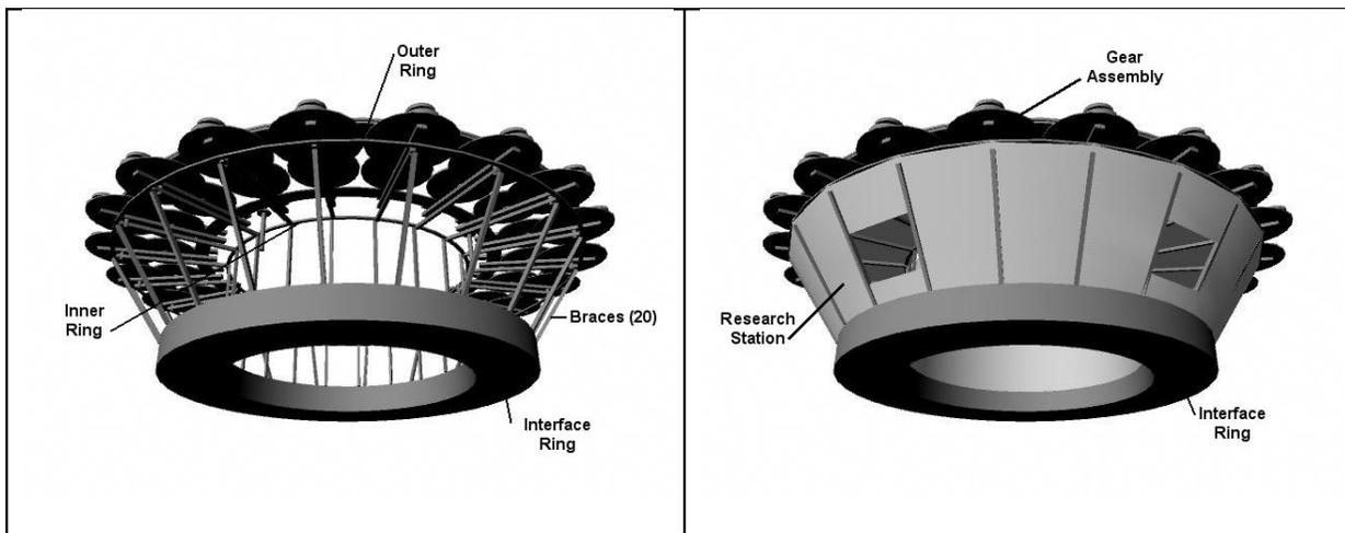
Figure 8. Turntable and Gear Assembly Support
