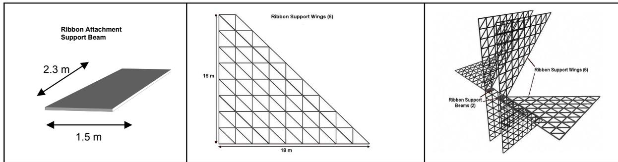
Figure 3. Ribbon Support Structure
