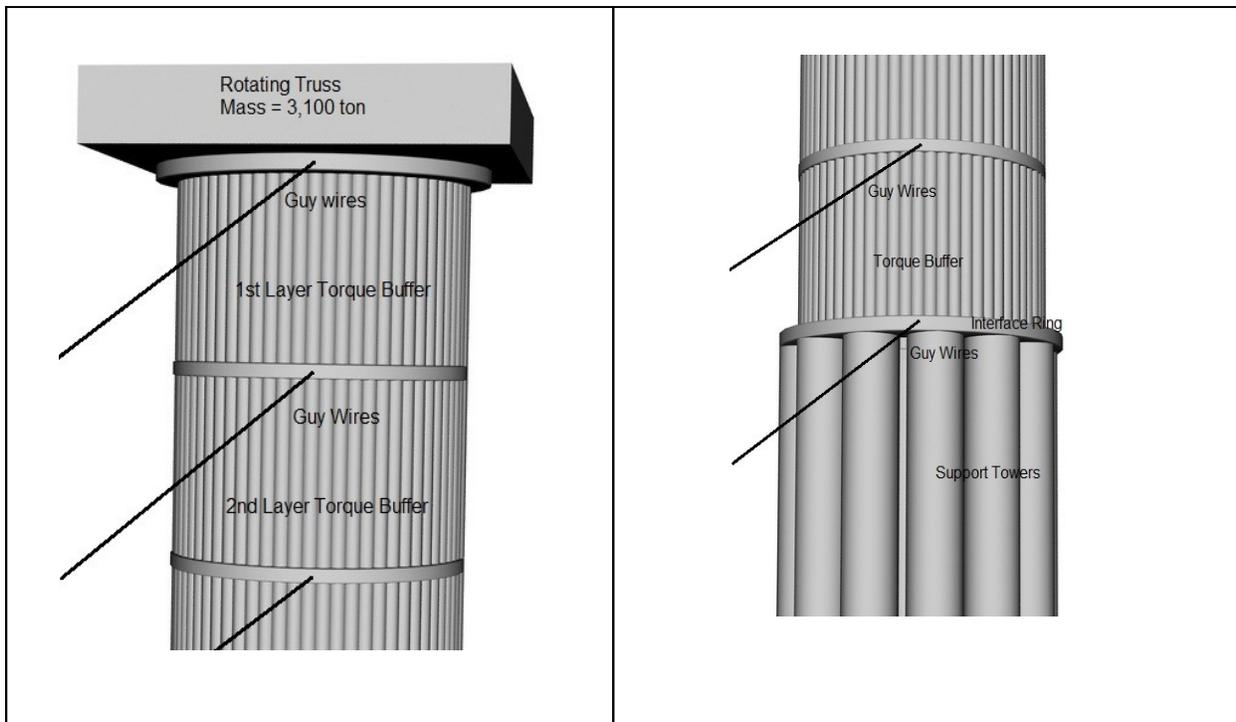
Figure 11. Torque Buffer & Support Towers
