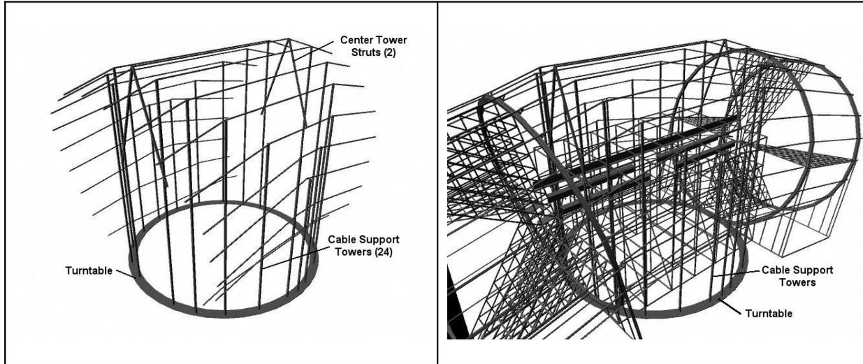
Figure 6. Cable Supports and Turntable
