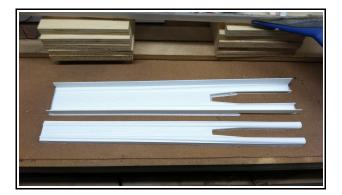
Also this month, I continued to design and print new canopy molds (2<sup>st</sup> picture). I plan on using a bottom mold and a top mold. The fiberglass will be sandwiched between the top and bottom mold. This should result in a more uniform canopy with ventral nacelles.
