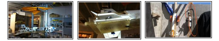
Also, this month, I attached the launch rail to rocket engine test stand and performed a dry run for launch. I used water as the propellant (pressurized to 40 psi) and ejected the canopy. Other than a few minor issues, the test run was perfect (i.e. I hit all the right buttons and it worked).
